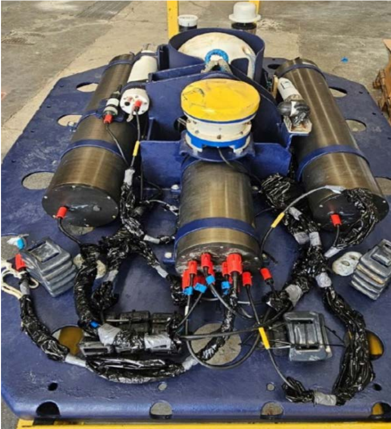
FIGURE 23: CCS LANDER USED FOR CONTINUOUS SEABED MONITORING
