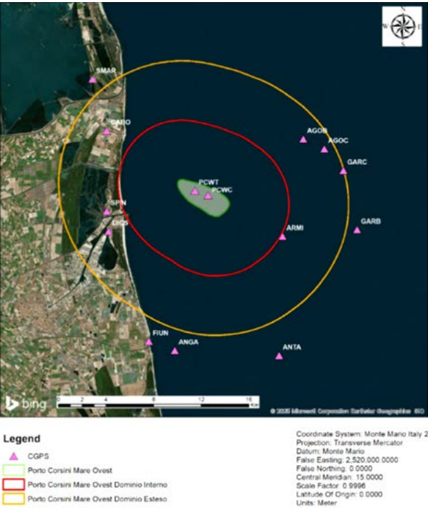
FIGURE 20: DISTRIBUTION OF THE CONTINUOUS GNSS MONITORING STATIONS WITHIN THE PROJECT AREA (left) LOCATION OF THE BENCHMARKS OF THE HIGH-PRECISION LEVELLING NETWORK (right)
